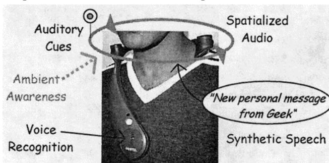
Figure 1: The primary wearable audio device, the *SoundBeam Neckset*. Messages are browsed in a unified manner via speech, auditory cues and spatial audio. The interface is controlled via voice and tactile input.
