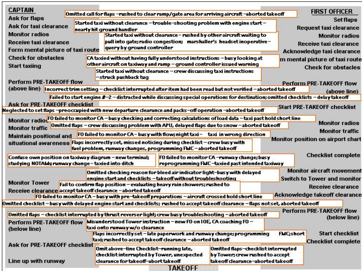
Figure 1. Errors associated with concurrent task demands reported to the ASRS. The left and right columns (grey) describe, from top to bottom, the flow of prescribed taxi activities for each of the crew members. The overlaid boxes (white) contain information about the error, the contributing factors, and the resulting outcome for each of selected incident reports.
