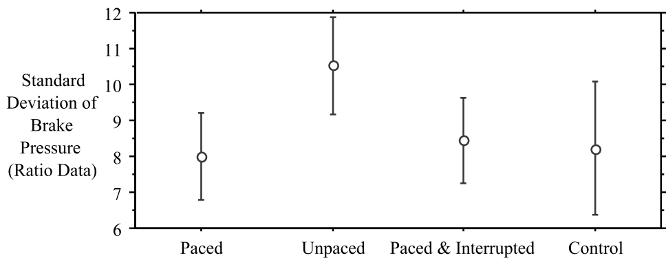
Figure 4. Summary of brake pressure by task type (error bars indicate 95% confidence interval for the mean).
