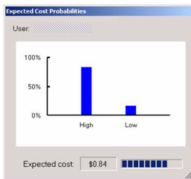
Figure 3. Real-time inference with BusyBody models showing probability distribution and expected cost of interruption for a user.
