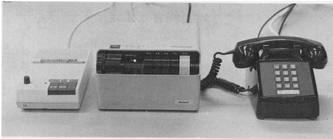
Fig. 1 The telephone system showing (from left to right) the handsfree unit, the telephone recording and announcing device, and the digital dial telephone.
