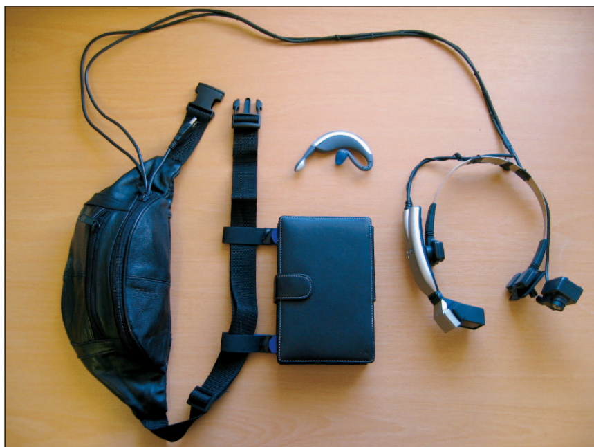
Figure 1. Wearable computer outfit: battery pack and VGA converter for the head-mounted display (left), U70P computer (lower center), Bluetooth headset (upper center), and M2 head-mounted display (right).
