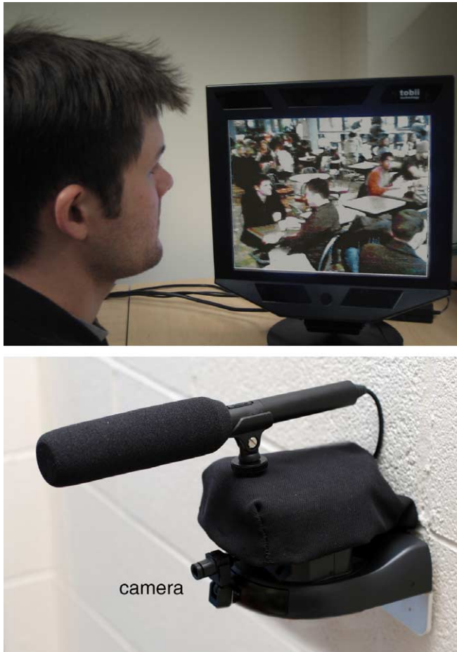
Fig. 11. OverHear eye tracking surveillance display (top) and robotic shotgun microphone (below).
