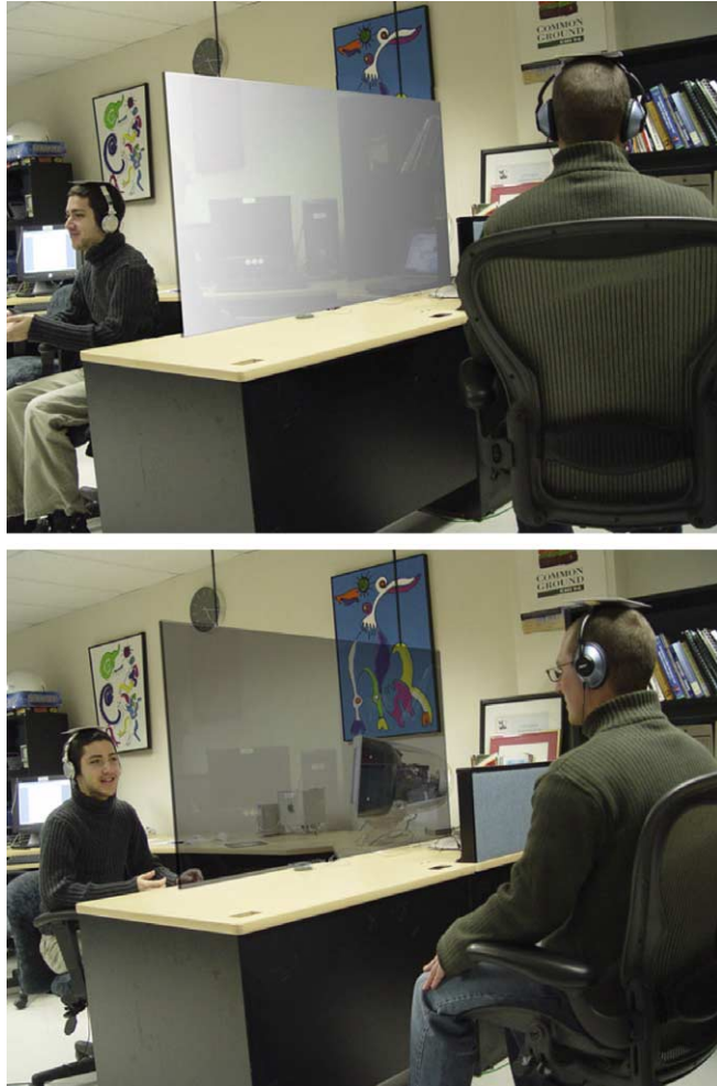
Fig. 10. Attentive office cubicle prototype in opaque (top) and transparent mode (bottom).
