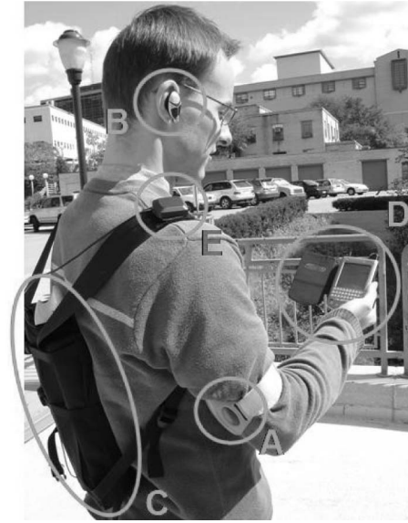
Fig. 5. Wearable Platform for current SenSay prototype: (A) SenseWear armband, (B) BlueSpoon headset, (C) backpack encompassing LifeBook P-1120 with 802.11b transceiver, (D) Tungsten W smart phone, and (E) external antenna for GPS receiver. The SenseWear armband is worn in contact with the skin and normally hidden from view.
