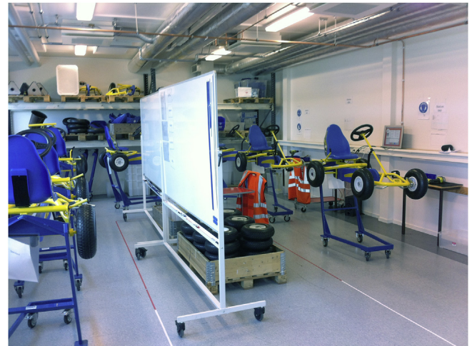
Fig. 1. The environment for the experiment seen from the same point as the video recordings. The assembly station and touch screen can be seen, as well as the cars awaiting assembly. The computer system and assembly station can be seen on the right side of the picture, and the disassembly station can be seen on the left side.
