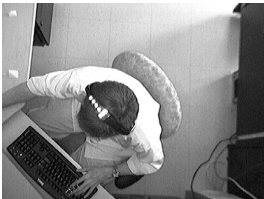
Figure 2. Retroreflective markers on people’s headsets ease the motion capture process.
